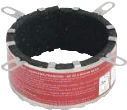
4hr Fire Collars Intumescent Fire Collars - 4 Hour Rating Fire rating: tested to BS476 Part 20 for 4 Hour in vertical / horizontal application. Code Size Pack Qty FC4H110 110mm Pack of 1
